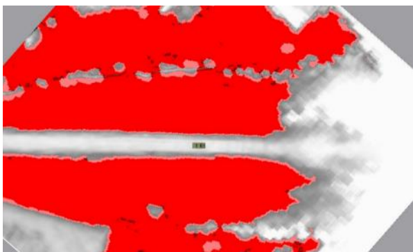
Figure 11: Slope magnitude map for test environment with negative slopes
