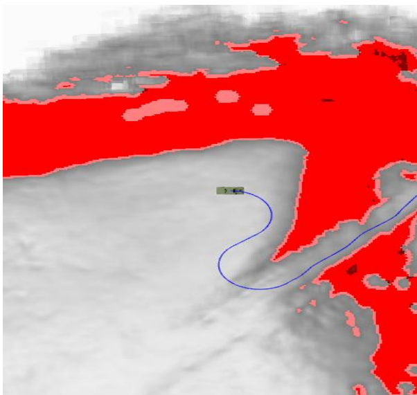
Figure 14: Slope magnitude map and Maverick plan to avoid lethal slope
